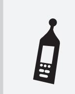
Sound waves are usually measured as root-mean-squared pressure in Pascals (Pa).
